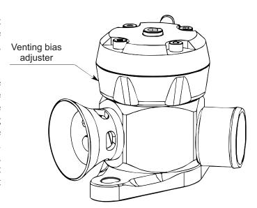
Typically, most un-modified engines will allow 100% atmosphere venting with no problems. However, some combinations of modifications can result in backfiring if high proportion of atmosphere venting is used, in which case the solution is simply to dial back the amount of air vented to atmosphere until the problem is resolved—this is one of the key benefits of the venting bias adjustment feature.
